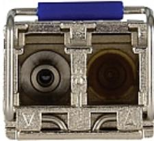
OSP-SM10 is a fiber optic transceiver for 1310nm single-mode signals. This standard pluggable SFP+ module has two LC connectors for reception and transmission signals over two strands of single-mode optical fiber
